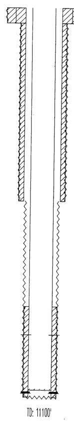
0.0 - 440.0' 17 1/2" OD HOLE 0.0 - 440.0' CEMENT 420sx-CIRC 0.0 - 440.0' 13 3/8" OD SURF CSG
