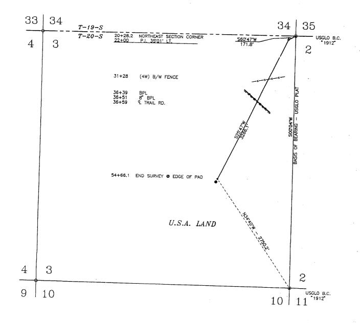
DESCRIPTION A STRIP OF LAND 50.0 FEET WIDE AND 3437.9 FEET OR 0.651 MILES IN LENGTH AND BEING 25.0 FEET LEFT OF AND 25.0 FEET RIGHT OF THE ABOVE CENTERLINE SURVEY.
