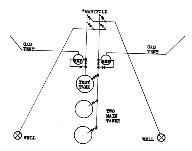
\*Note:- Manifold used to switch either thru the test separator into the test tank.
