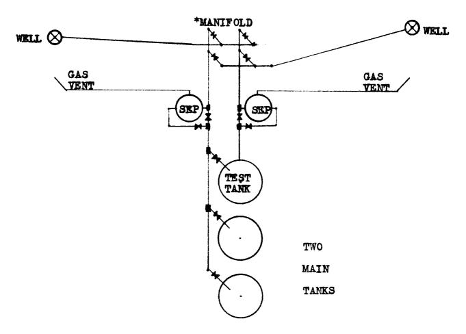
\*Note: - Manifold used to switch either well thru the test separator into the test tank.
