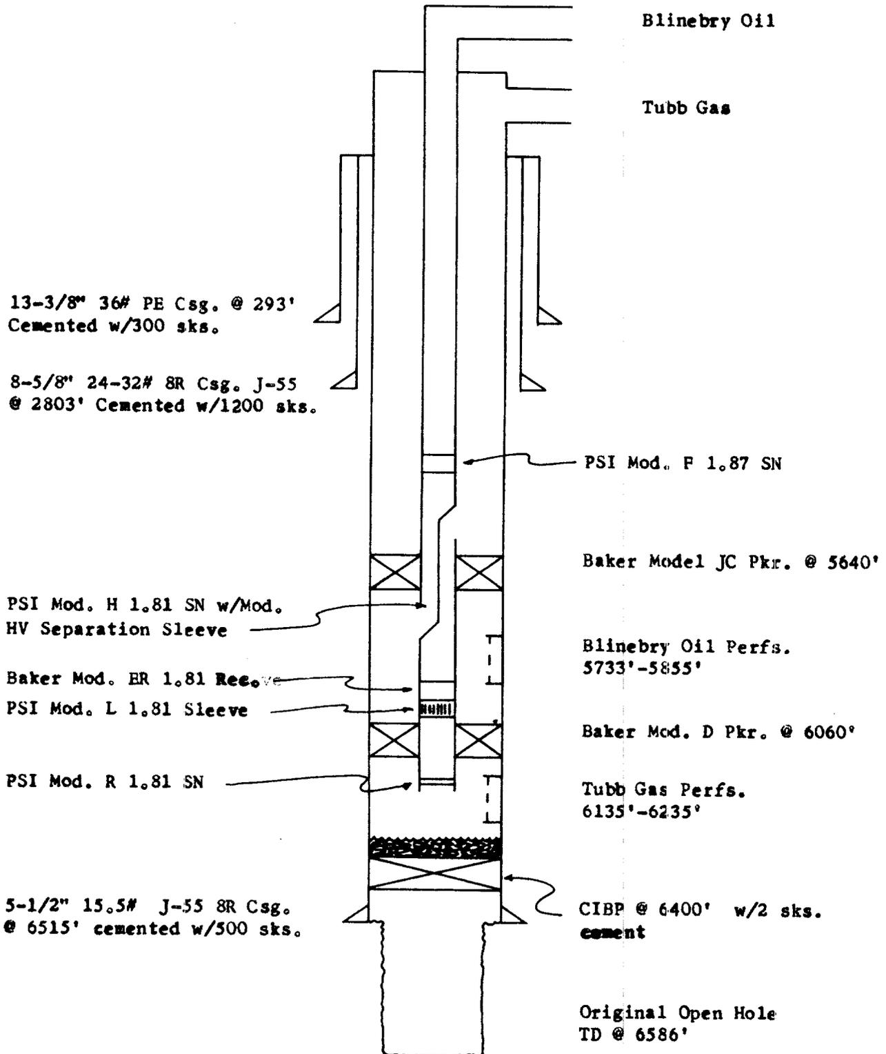
NOTE: No temperature survey available. Cement behind 5 1/2" casing calculated to 3200'. Cement volumes on 13-3/8" & 8-5/8" calculated to circulate.
