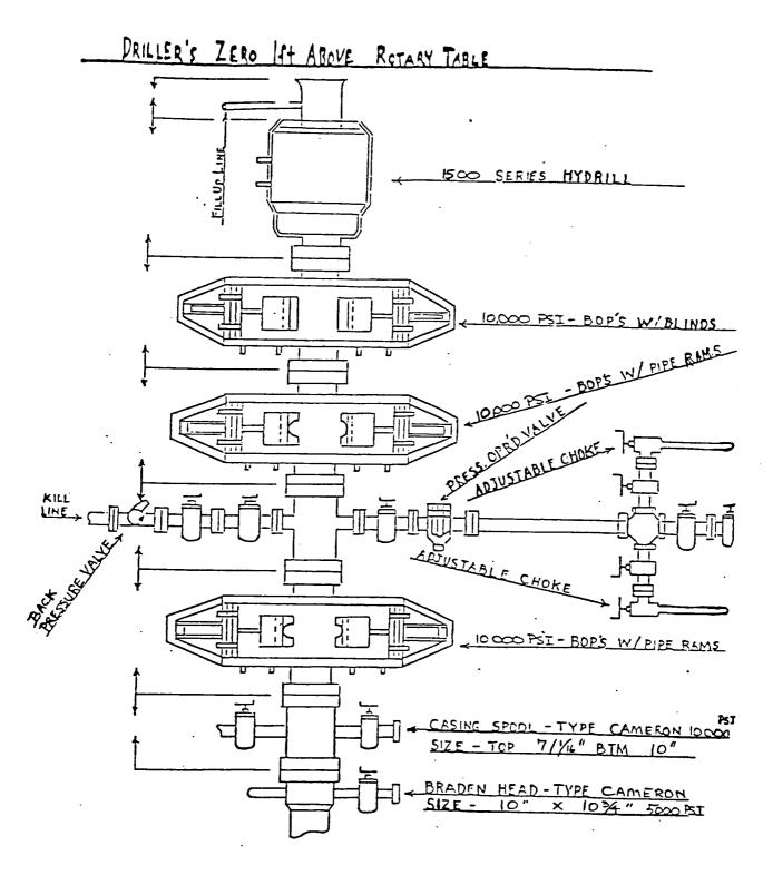
BOP HOOK UP AFTER SETTING SURFACE (1034") + INTERMEDIATE (75%) STRINGS. ALL CONNECTIONS FROM THE SPOOL UP WILL BE TESTED TO 10,000
