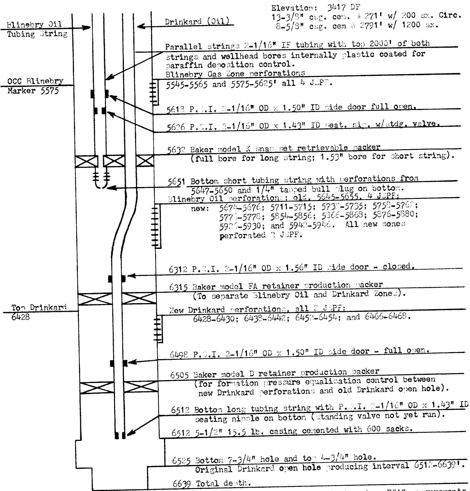
**Note:** All tubular and packer depths based on PGAC measurements in setting FA and D Baker packers.
