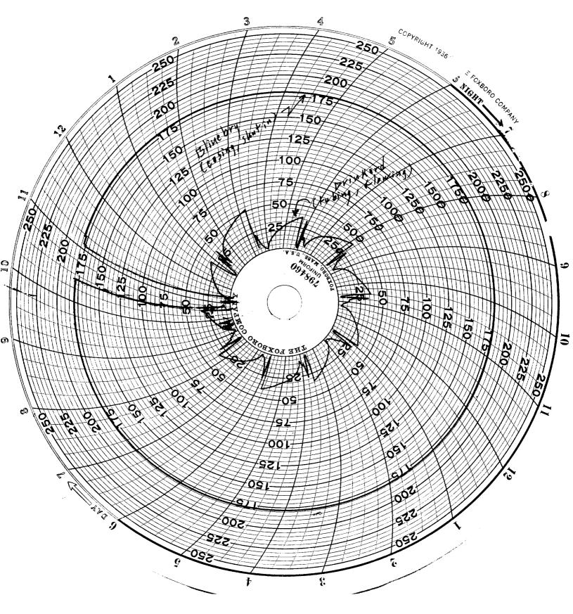
Markhom, Cone & Redfern Dist Drinkard Lease Eubanks Well No. Dare On 5/2 Time On Winds Time off Wind Length of Test nights. Chicke Size \_\_\_\_ Line Size \_\_\_ Orifice Size \_\_\_ Beg Gauge End Cauge Taken by\_ . Approved Blue line = Drinkerd (flowing by pressure - time
