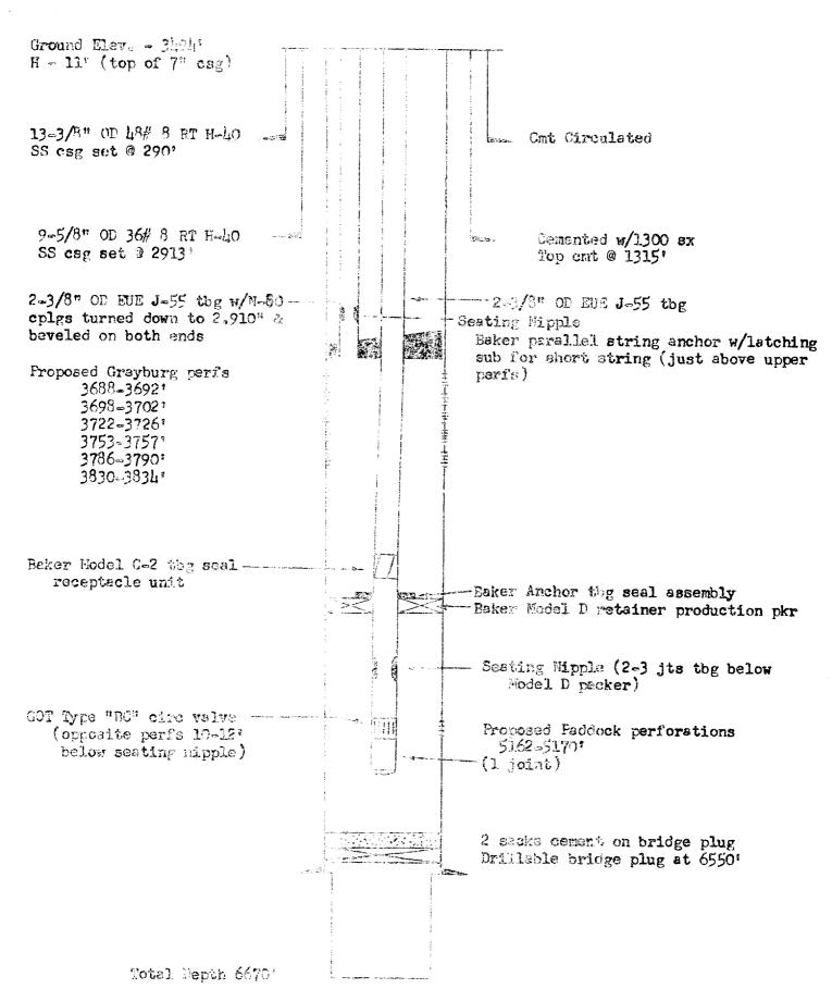
DIAGRAPMATIC SEFTCH OF MECHANICAL INSTALLATION PADDOCK - PENEOSE SEELLY, OTL-OTL DUAL GULF OIL CORPORATION - C. A. HARDY NO. 4
