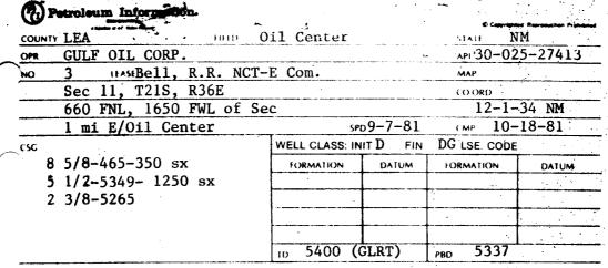
IP (Glorieta) Perfs 5232-61 F 1400 MCFGPD. Pot based on 24 hr test thru 43/64 chk. GOR Dry; gty (Gas) (NR); CP Pkr; TP 70
