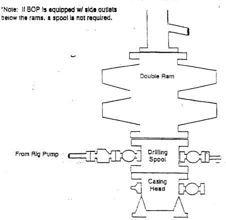
2 000 psi WP Double Ram Blow-out Preventor. Must be tested to 1000 psi prior to drilling out 8-5/8° surface casing.
