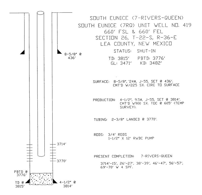
HISTORY: DRILLED IN AUGUST, 1961. COMPLETED IN QUEEN F/3714'-3770'. F/20000 GALS DIL & 30000# SD. INSTALLED GAS LIFT & A/30000 SCF N2 PAD & 500 GALS MUD ACID & 2000 GALS TREATED LEASE DIL W/26150 SCF N2 IN MARCH, 1962. INSTALLED PUMPING UNIT. SHUT-IN NOVEMBER, 1990 AFTER PRODUCING 35 MBD, 39 MMCF, & 48 MBW FROM 7-RIVER-QUEEN.
