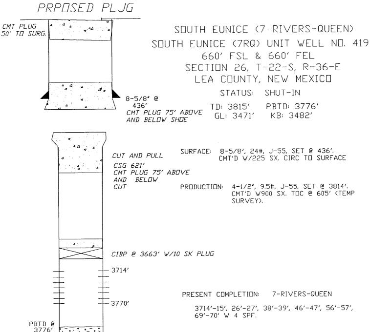
HISTORY: DRILLED IN AUGUST, 1961. COMPLETED IN QUEEN F/3714'-3770'. F/20000 GALS DIL & 30000# SD. INSTALLED GAS LIFT & A/30000 SCF N2 PAD & 500 GALS MUD ACID & 2000 GALS TREATED LEASE DIL W/26150 SCF N2 IN MARCH, 1962. INSTALLED PUMPING UNIT. SHUT-IN NOVEMBER, 1990 AFTER PRODUCING 35 MBD, 39 MMCF, & 48 MBW FROM 7-RIVER-QUEEN.
