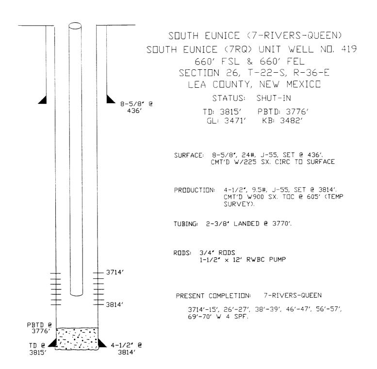
HISTORY: DRILLED IN AUGUST, 1961. COMPLETED IN QUEEN F/3714'-3770'. F/20000 GALS DIL & 30000# SD. INSTALLED GAS LIFT & A/30000 SCF N2 PAD & 500 GALS MUD ACID & 2000 GALS TREATED LEASE DIL W/26150 SCF N2 IN MARCH, 1962. INSTALLED PUMPING UNIT. SHUT-IN NOVEMBER, 1990 AFTER PRODUCING 35 MBD, 39 MMCF, & 48 MBW FROM 7-RIVER-QUEEN.
