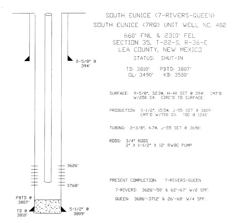
HISTORY: DRILLED IN AUGUST, 1957. COMPLETED IN QUEEN F/3686'-3768'. A/500 GALS. F/10000 GALS GELLED LEASE DIL & 10000# SD. INSTALLED GAS LIFT IN MAY, 1961'. INSTALLED PUMPING UNIT IN DCTOBER, 1974. ADDED PERFORATIONS IN SEVER RIVERS F/3626'-67' IN NOVEMBER, 1990. A/3000 GALS. COULD NOT PUMP OFF BOTH ZONES (100% WATER). SET RBP @ 3680'. TESTED ALL WATER. RETREIVED RBP IN JUNE, 1991. SHUT-IN AUGUST, 1991 AFTER PRODUCING 62 MBD, 66 MMCF, & 266 MBW FROM 7-RIVERS-QUEEN.
