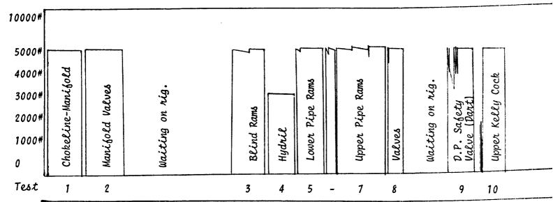
The above is a transposition of the pressure recorder chart covering test to the blowout control equipment in service on your well drilling in the Jal, New Mexico Area, Midland District, Texas. Test was made with test plug landed in casing head with the following test results: Arrived location - rig coming out of hole.
