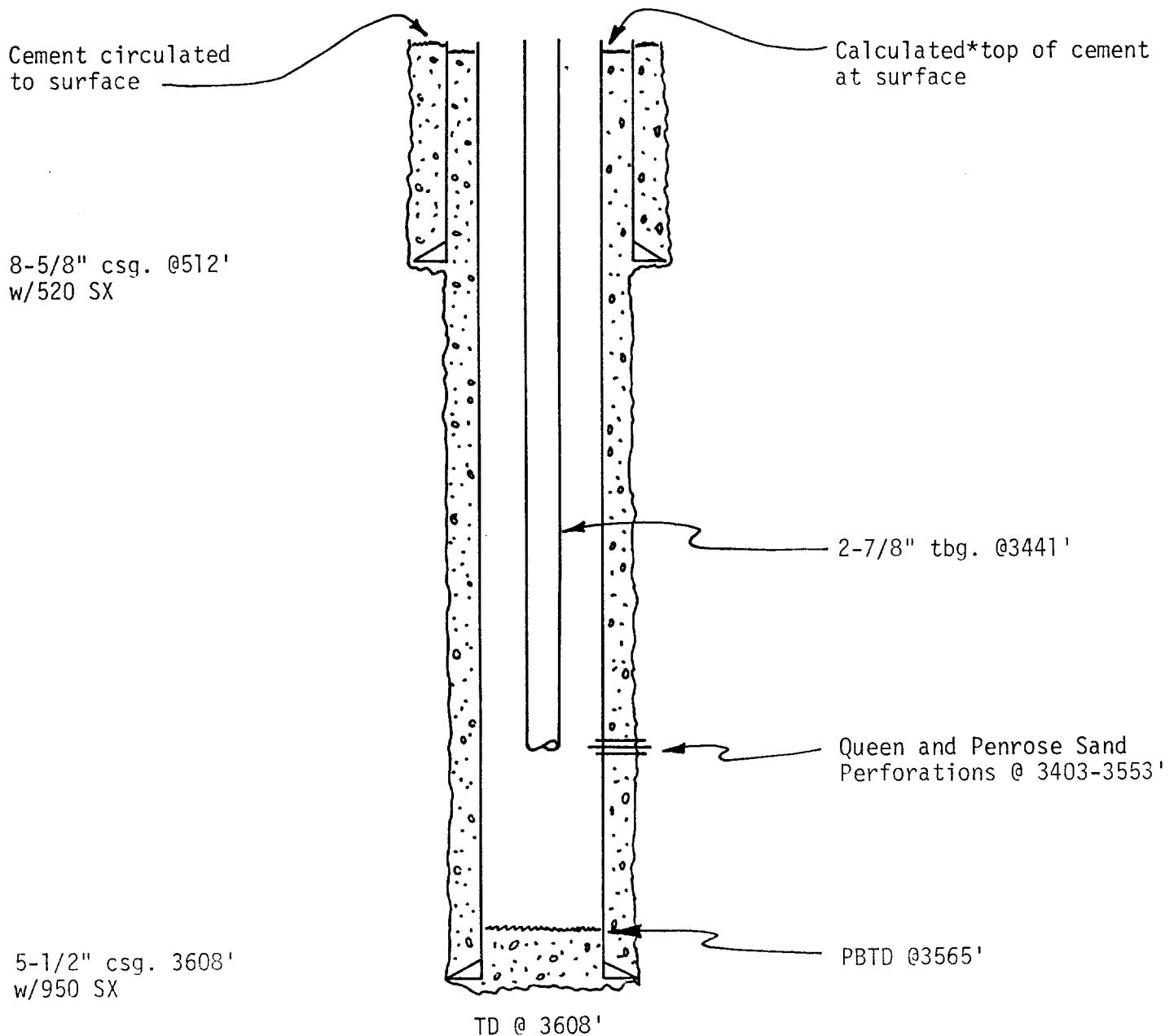
\* Theoretical calculation based on hole size, sacks of cement used, and a yield of 1.18 cubic feet of fill per sack of cement.
