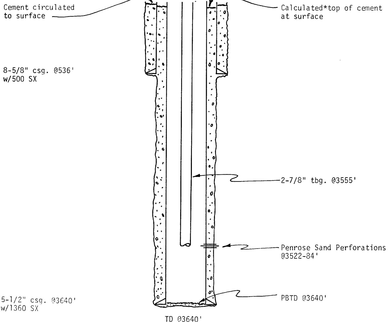
\* Theoretical calculation based on hole size, sacks of cement used, and 1.18 cubic feet of fill per sack of cement.
