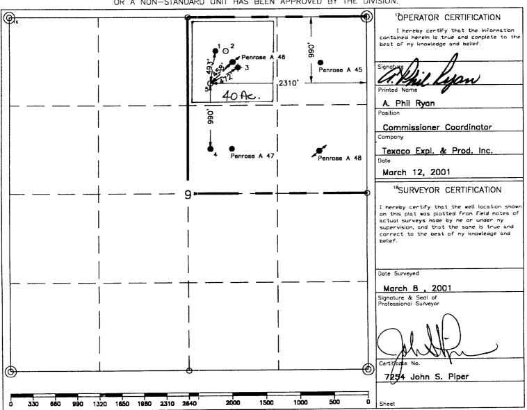
$\bigcirc$  = Staked Location  $\bullet$  = Producing Well  $\not$  = Injection Well  $\cdot \diamond$  = Water Supply Well  $\cdot +$  = Plugged & Abandon Well
