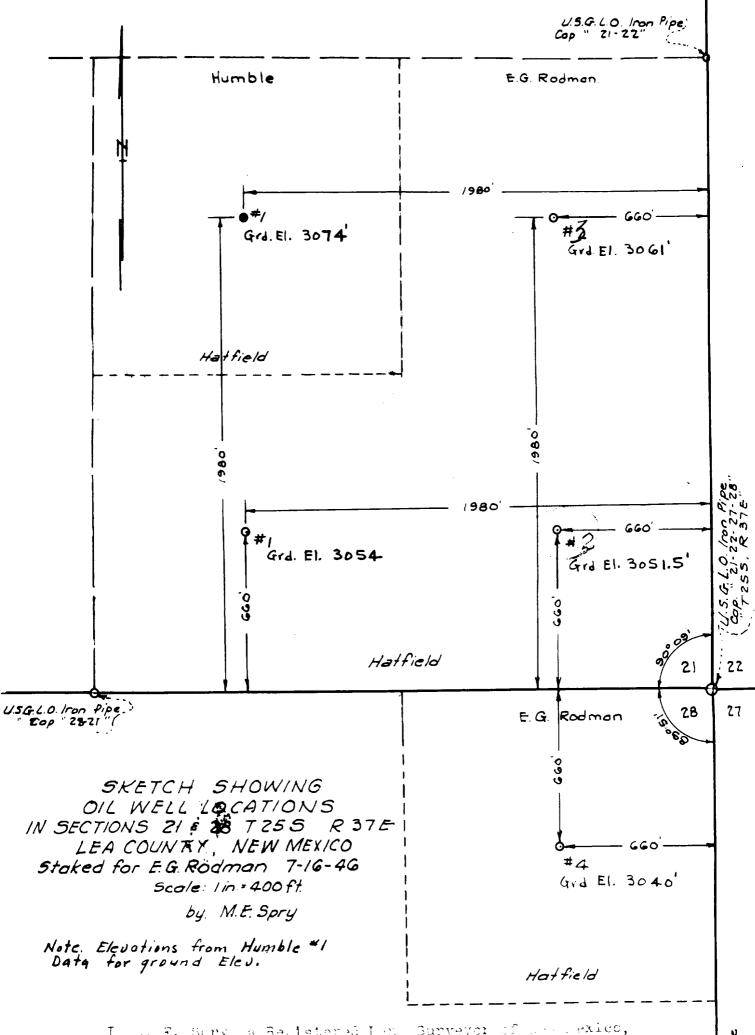
I, ... E. Sery, a Resistered Lyn. Surveyor of the exico, hereby certify that the alove plat represents and of the survey make by me upon the ground on the SE & Section Ol and on the NE% of Section 28, both in TOSS RY7E. Les County les exico. Surveyed July 16, 1946.
