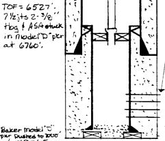
N-80 (6828-23 16 J-55 (5290-0'). a + 5955": Cemented w/ 465 sx cement, TOC= 3350'(15 "15.5 16 5-55 Imer set at 69% 5½" x7" TIW hanger at 6730(TOL) Cemented w/ 65 sx cement TOC= 6730
