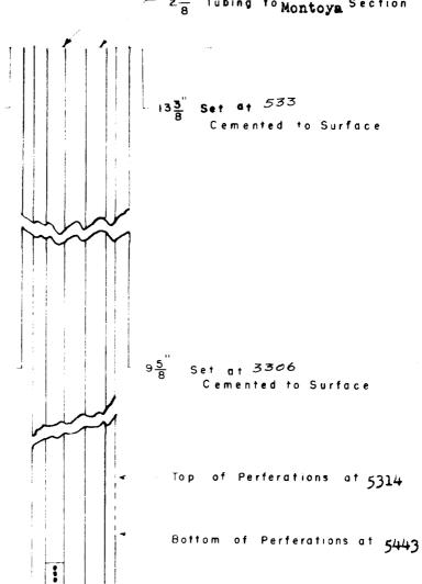
Tubing for Blinebry Section Set in Baker Parallel Tubing Anchor at 5524
