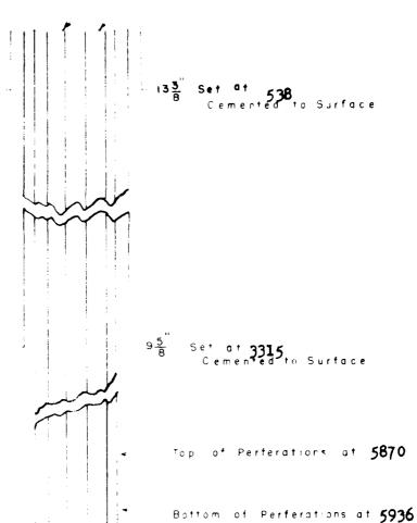
Tubing for **Drinkard** ection Set in Baker Parallel Tubing Anchor at **6026**
