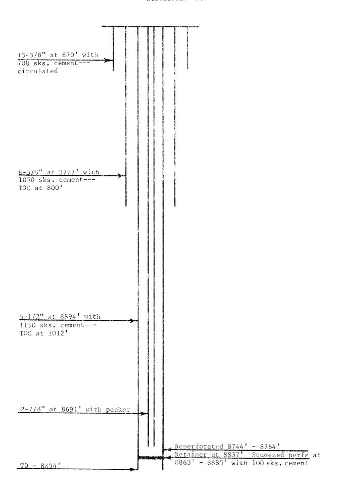
Well was originally drilled in 1978 to the Crosby Fusselman formation. PBTD at 8775.
