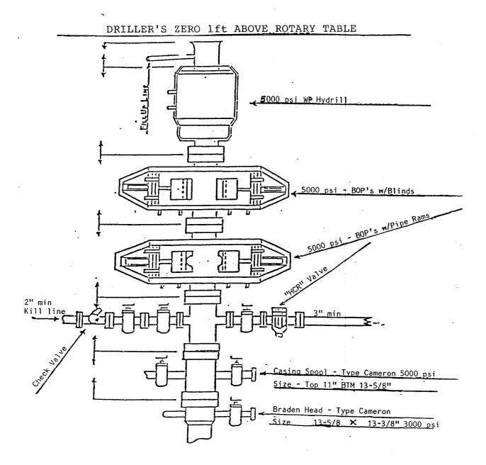
BOP HOOK UP AFTER SETTING INTERMEDIATE (8-5/8) STRING. ALL CONNECTIONS FROM THE SPOOL UP WILL BE TESTED TO 5000 psi.
