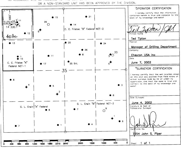
$\bigcirc$  = Staked Location • = Producing Well  $\checkmark$  = Injection Well  $\diamond$  = Water Supply Well  $\overset{\bullet}{\bullet}$  = Plugged & Abandon Well
