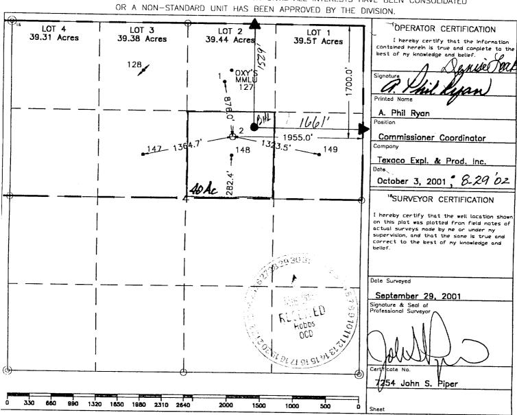
🔾 = Staked Location • = Producing Well 🎤 = Injection Well 💠 = Water Supply Well 💠 = Plugged & Abandon Well  $\bigcirc$  = Found Section Corner, 2 or 3" Iron Pipe & GLO B.C. O = Found /4 Section Corner, 1" Iron Pipe & GLO B.C.
